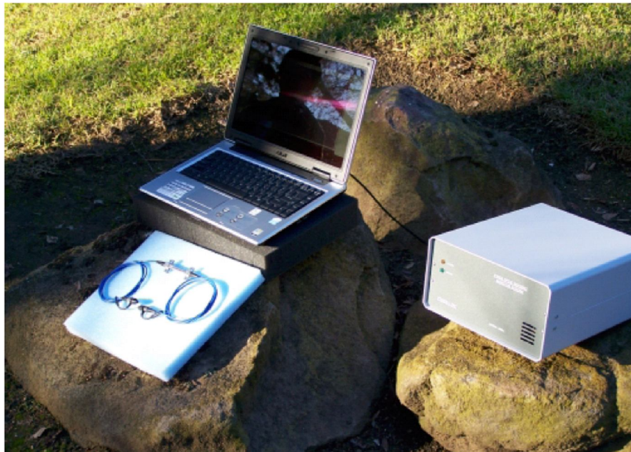
Figure 2. Fibera 2000A Fiber Optic Sensing Monitor System
